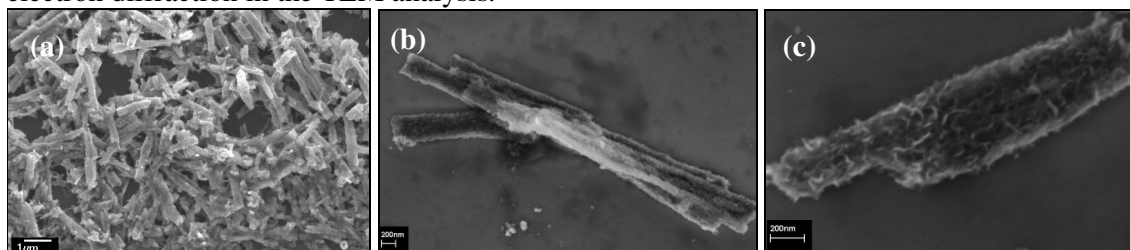
Figure 1 – HRSEM images obtained for the NdNiO 3 nanotubes.
